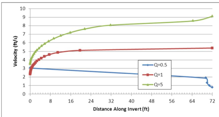
Based on this analysis of a simple smoothbore concrete pipe, we conclude that passage can only be reliably achieved when tides are at or above the inlet (22%); hydraulic analysis indicates that passage is not likely when tides are in the pipe (25%) due to conditions depicted in Figures 9 and 10. Passage is physically impossible when tides drop below the outlet (53%) and therefore is not under consideration.
