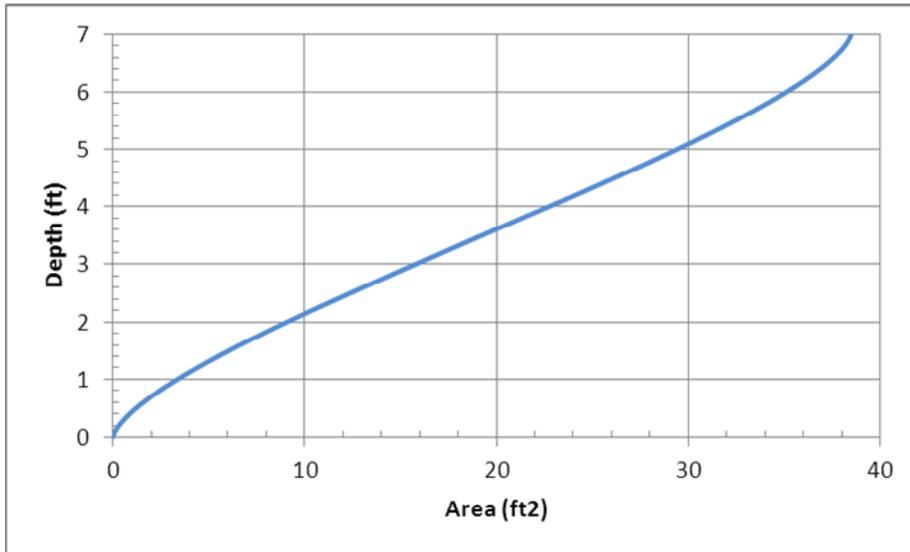
Figure 8. Circular geometry – surface top width as a function of depth (D = 7')
