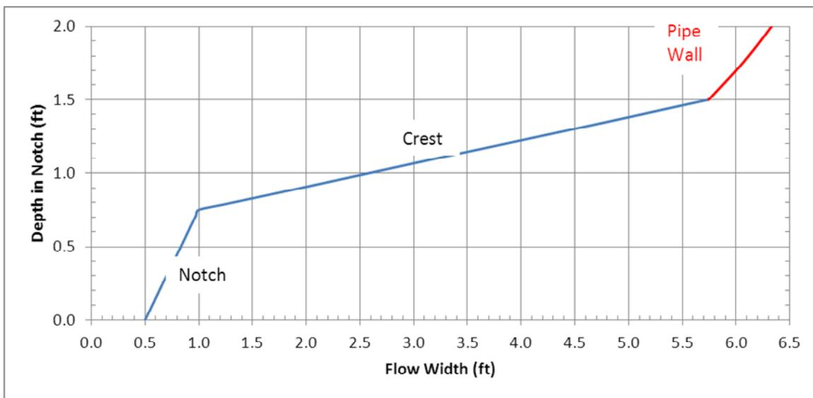
**Figure 13. Weir Flow Area Function**
