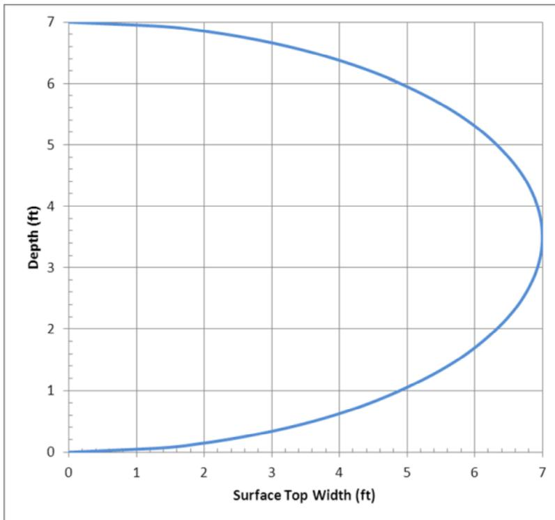
The combination of steep pipe ( $S = 0.042$ ) and smoothbore material (concrete;  $n = 0.012$ ) would suggest that alewife can only pass when tidal stage submerges the inlet invert; in other words, when the pipe is completely backwatered. Otherwise flow depths can be too shallow ( $< 4'' = 0.33'$ ) and/or velocities too fast ( $> 5$  ft/s). This is confirmed by calculations with the HY-8
